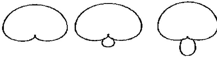
Figure 6. Cardioid, supercardioid and hypercardioid polar response patterns.
